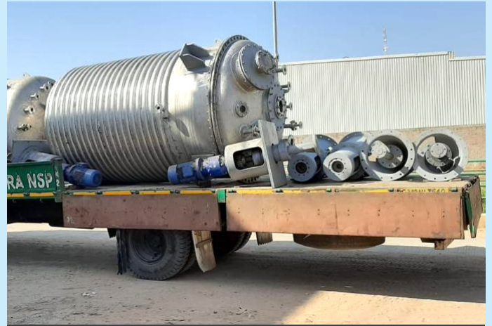
LIMPET COIL VESSEL AND JACKETED VESSEL
