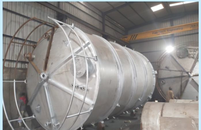
ALUMINUM STORAGE TANK
